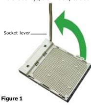
When the CPU is in place, push down the socket lever to secure the CPU. The lever clicks on the side tab to indicate that it is locked.
